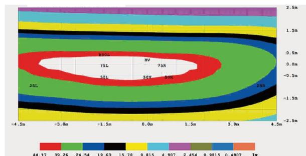
Height of Lamp Fixed: H = 1.00m Illumination Area) : L = 200.0 m ,W = 20.0 m Voltage : 12.00V Current : 2.625A Power : 31.5W
