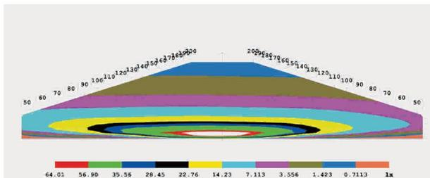
Height of Lamp Fixed: H = 1.00m Illumination Area) : L = 200.0 m ,W = 20.0 m Voltage : 12.00V Current : 2.625A Power : 31.5W
